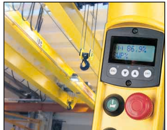
Safe Working Period calculation and condition monitoring for optimal maintenance .
